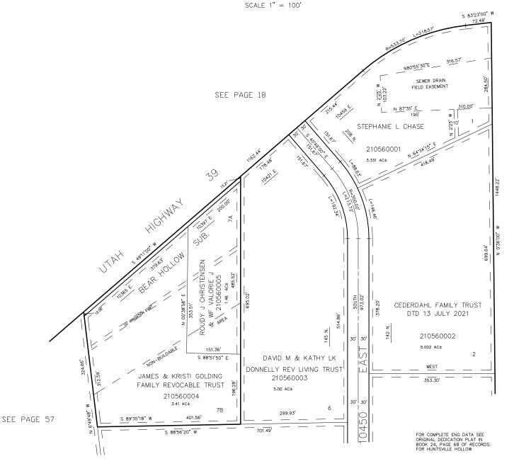
10' UTILITY & DRAINAGE EASEMENTS EACH SIDE DF PROPERTY LINES AS INDICATED BY DASHED LINES EXCEPT AS OTHERWISE SHOWN.
